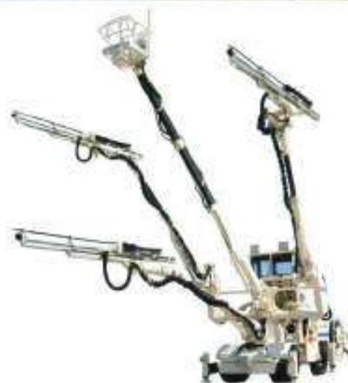
T3RW-210 Wing Boom Yoke Type With HD210 Hydraulic drifter
