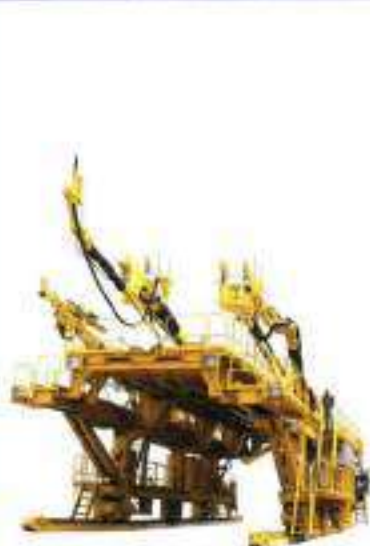
Tunnel Work Station (TWS) Self-propelling 2-boom with concrete sprayer.
