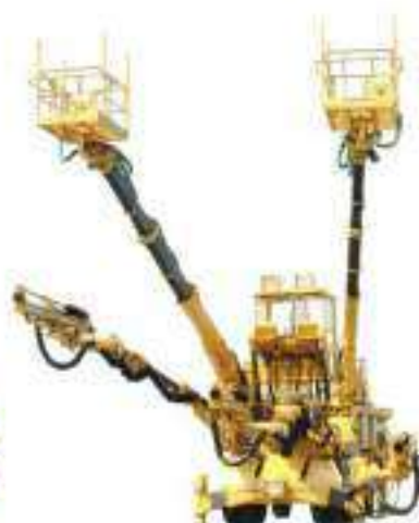
JTH3200R 3-boom, 2-cage Wheel Jumbo With HD210 Hydraulic drifter.
