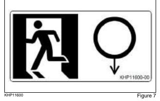
This decal shows that in an emergency you have to pull the ring on the back window seal in order to force open the rear window to make an emergency exit from the machine.
