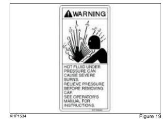
This decal warns the operator to wait and relieve pressure before opening the radiator cap.
