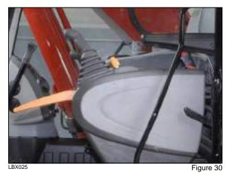
In the lowered position, all hydraulic controls are operational.
