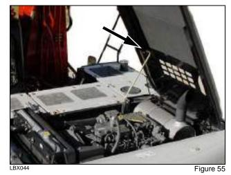
To close, push the hood up and slide the bar forward to unlatch the hood stay.
