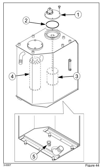
Replace the suction filter (3) and the return filter (4). See Cleaning and replacement of the suction filter and Return filter replacement on the previous page.
