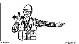
TURN EXCAVATOR RIGHT (SWING LOAD RIGHT) To stop movement, stop moving hand and clench fist.
