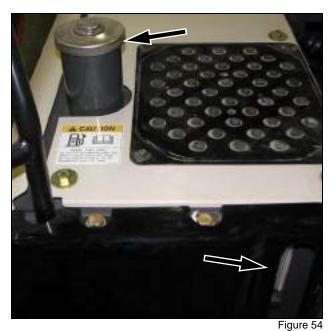
There is a sight gauge on the outside to check the level of the fuel in the tank.
