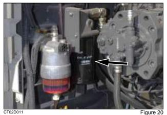
6. Coat the seal of the new filter with a fine film of oil.
