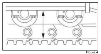
7. Measure the slack between the base of the undercarriage and the upper part of the track tread. See Track Tension Value on the next page.
