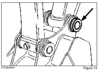
4. Start the engine. Remove the bucket cylinder rod to bring it in its housing, shut down the engine and remove the starter switch key.
