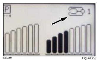
When you select either crusher (1) or breaker (2) mode it is displayed on the monitor. In figure 29 crusher 1 is the mode the machine is in.
