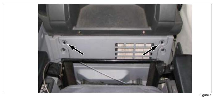
To access the fuses, remove the cover of the box.
