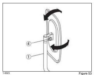
WARNING: When transporting the machine make sure the mirrors are not protruding from the machine. Fold the mirrors inward to avoid an accident.
