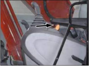
3. Make sure the engine throttle button is in low idle position.
