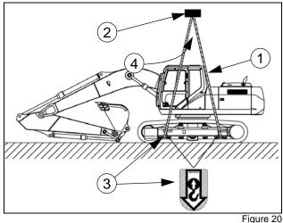
2. Use a wire rope with a sufficient strength for lifting, and route the wire thru the lifting points(3). Use a supporting bar (2) that will keep the rope away from the machine. Make sure the lifting angle(4) is between 30° and 40°.
