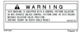
This decal warns the operator of the control patterns selector valve and that there are two different control patterns. It is best to check the controls in an open area to make sure the controls match the card in the window.
