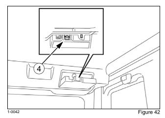
4. Raise the windshield and press it into the Auto-lock (4) located in the rear left portion of the cab roof to securely fasten the windshield. Keep your hands on the handles until it has been engaged into the auto-lock. Push the windshield back and forth to make sure it is secure in the Auto-Lock.
