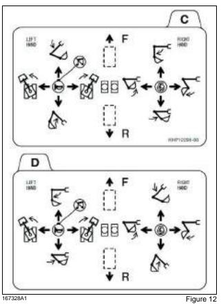
This card located on the cab window shows both of the configurations of the controls. Before operating the machine it is best to check the controls in an open area.
