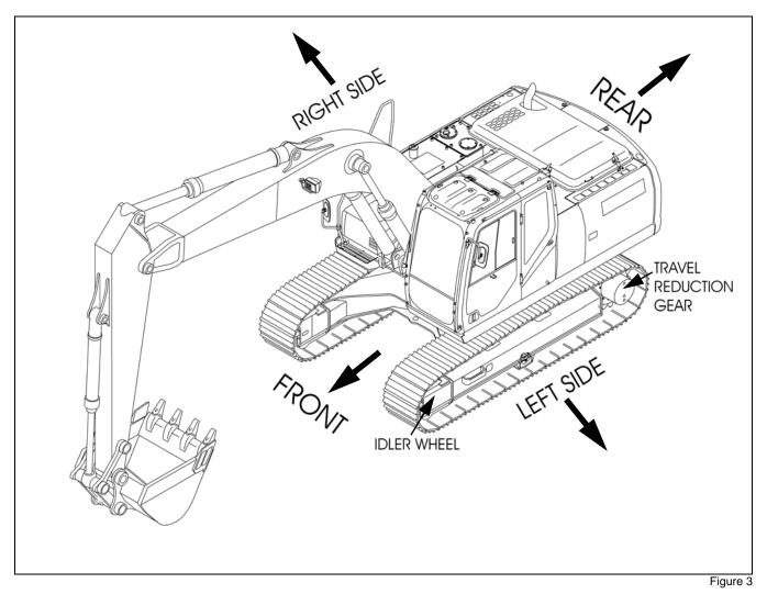
The terms Right-hand, Left-hand, Front, and Rear are used in this manual to indicate the sides as they are seen from the operator's seat when the cab is over the idler wheels.
