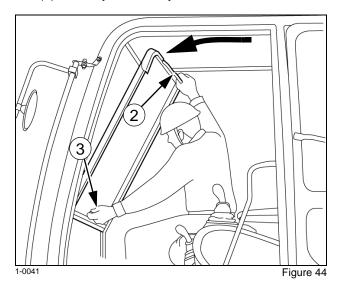
3. When the windshield is completely lowered press top handle (7) the top of the windshield.
