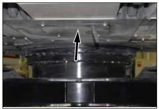
4. Remove the cap (2) and place a receptacle under the machine, connect the oil drain hose (3) to the green plug (4). When the hose is connected the oil will start to flow out the oil drain hose.
