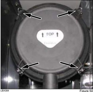
2. Remove the outer element.
