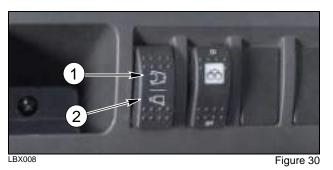
When the rocker switch is pressed again you will be in a different mode and it will display what the maximum flow is. There are 5 different settings for the crusher and the breaker.
