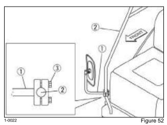
2. Loosen the bolt (4) and attach the mirror to the stay(1).
