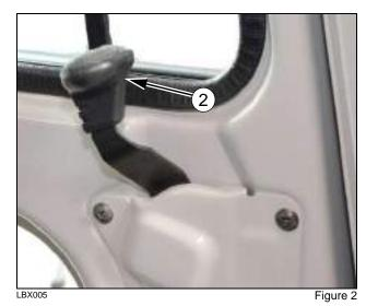
The door can be latched in completely open position. To unlatch the door, push the lever (3) downward.
