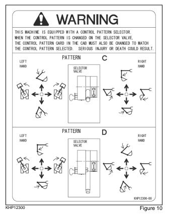
This decal shows the two different patterns that the controls can be adjusted to. If you switch the control pattern be sure to change the control pattern card in the cab.
