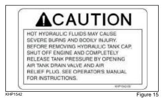
This decal warns the operator of the hot hydraulic fluid that can cause burns if the pressure in the tank is not properly relieved. Further instructions are located in maintance section.
