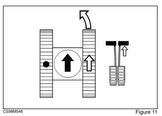
Turning to the right (Forward Travel) Simply press the left-hand pedal or the left-hand lever forward.
