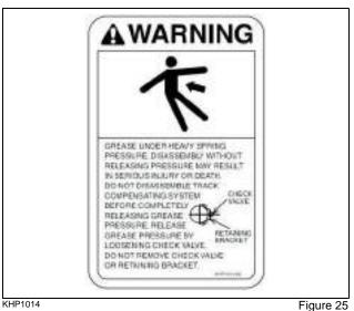
This decal warns the operator to release the pressure on the track assembly before disassembly.
