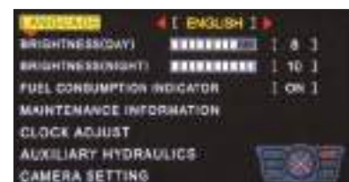
From the Computer Menu, you can change the monitor language, program service reminders and change auxiliary settings for flow to name a few.
