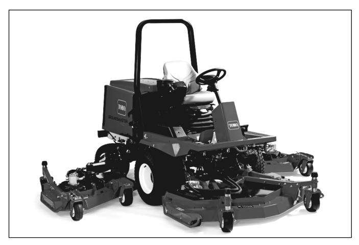
**MOUNTING:** Cutting decks are supported by lift arms controlled with individual lift switches.
