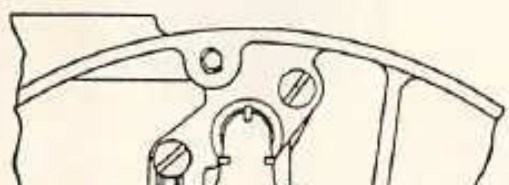
Fig. O78 — Using Ensign gage 8276 to set the fuel inlet valve lever to dimension "X" as indicated in Fig. O76.
