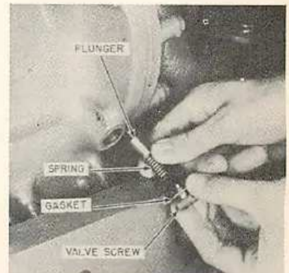
Fig. O66 — View showing main oil gallery relief valve.
