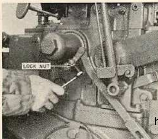
Fig. O145 — View showing lift link free travel adjustment.
