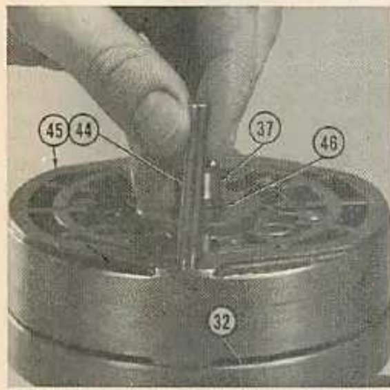
Fig. O39 — Removing dowel pins (44) from pump ring and rotor assembly (45) and housing (32). Discard snap ring (46) after it is removed from stub shaft (37) and install new snap ring on reassembly.
