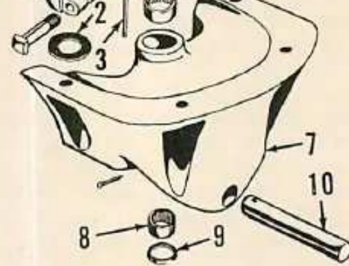
Fig. O7—Exploded view of Industrial front bolster for power steering equipped model. While shape of bolster or carrier differs for other models, operating parts remain basically the same for all axle type models with power steering.
