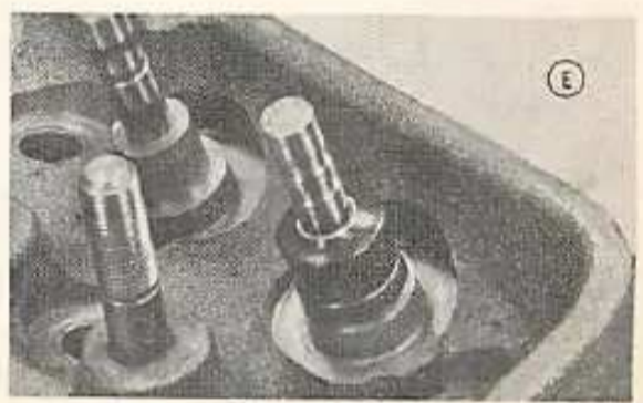
Fig. O58 — Views A through E illustrate method of installing Perfect Circle valve stem seals on models so equipped. Photos courtesy of Perfect Circle Corporation.
