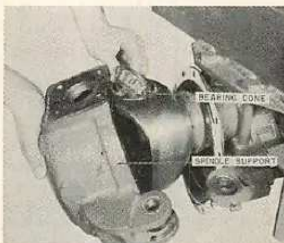
Fig. O22 — Remove spindle support from outer end of axle housing as shown.
