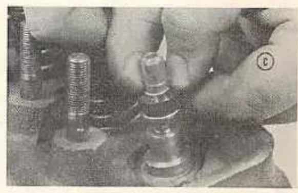
Fig. O57 — Cylinder head cap screw tightening sequence for Series 1600 diesel engines. Tighten the oil cap screw (24) to a torque of 96-100 Ft.-Lbs. and all other cap screws to a torque of 112-117 Ft.-Lbs.
