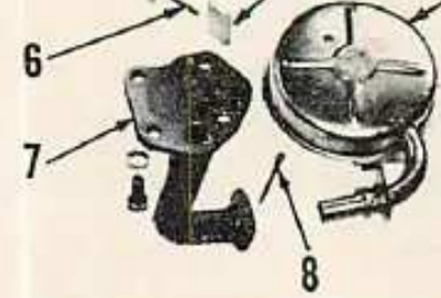
Fig. O62 — Exploded view of vane type oil pump used in all models except Series 1650 diesel.
