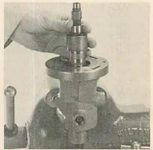
Fig. O43 — Removing the actuator assembly (stub shaft and control valve spool) from housing. Be careful not to cock spool in bore of housing.
