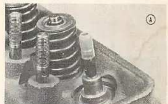
Fig. O55 — Cylinder head tightening sequence for Series 1650 diesel engines only. Tighten all capscrews to a torque of 129-133 Ft.-Lbs.
