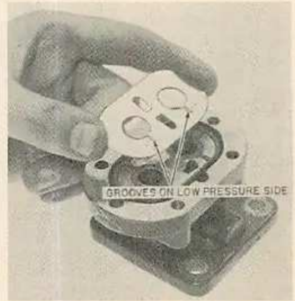
Fig. O28 — Install diaphragm with bronze side up and grooves towards low pressure side of pump as shown.
