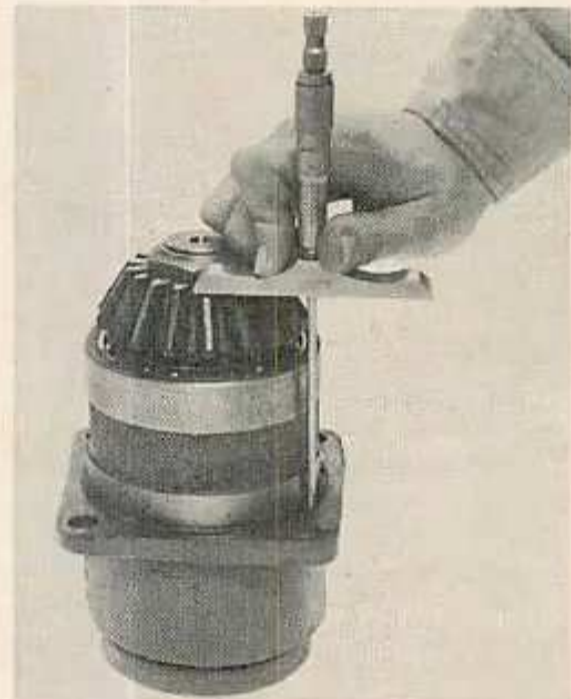
Fig. O132 — Measurement between points shown is used in determining thickness of shims to use for proper location of gear in housing. Refer to text for procedure.
