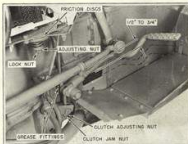
Figure 6-1 Clutch Pedal Adjustment
