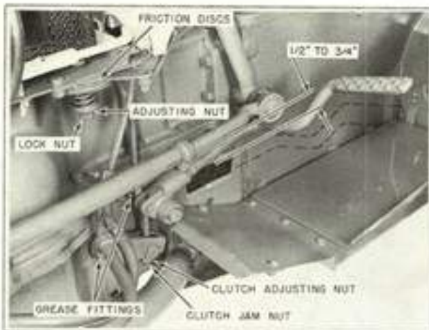
Figure 1-7 Clutch Pedal And Governor Control Friction Discs
