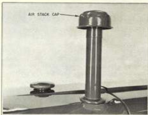
Figure 3-1 Air Stack Cap
