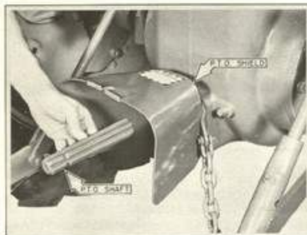
Figure 10-3 Installing Power Take-Off Shaft
