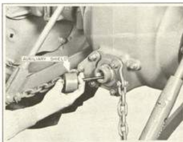
Figure 10-4 Installing Power Take-Off Auxiliary Shield
