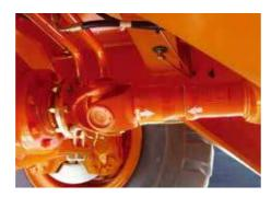
Transmission shaft: Apply reinforced transmission shaft and self-locking nuts are used as the connecting bolts of the transmission shaft so as to improve the durability of transmission system.
