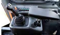
Pilot operating system provides comfortable machine control.
