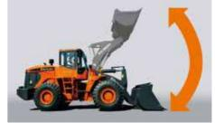
Arm Raise Kick-out and Return to dig function: reduce the intensity of your work and improve working efficiency.
