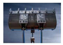
The diameter of the hinge pin in the 6 operating devices is 5-10mm larger than the level of the industry. High wear-resistant materials are used for pin sleeves so that the durability of working device is stronger and the residual value of second-hand equipment is higher after being coated with MoS2 and processed with a special heat treatment process.
