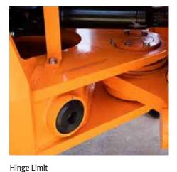
DISD loader adopts a new part - the nylon hinge limit block. It has stronger durability, no noise caused by impact and reduces the driver's fatigue.
