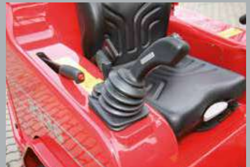
The slightly twisted joystick position simplifies operation.
