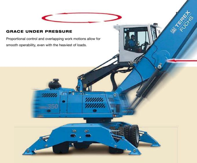
INNOVATIVE DUAL CIRCUIT HYDRAULIC SYSTEM PROVIDES BOTH HIGH PRECISION HANDLING AND FREEDOM IN WORK MOTIONS
