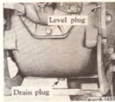
Illust. 40D Transmission oil level and drain plug.
