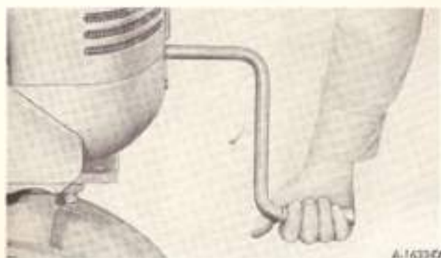
Illust. 12 Correct method of hand-cranking.
