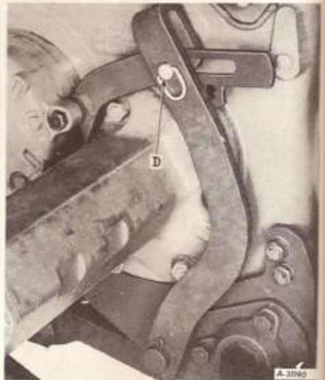
Illust. 24A Quick-attachable pin in position for implements with gauge wheels.
