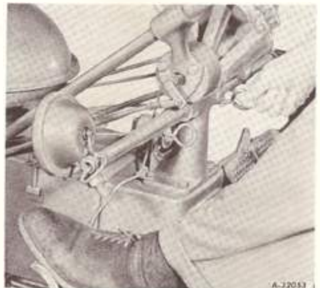
Illustr. 11B Pulling the starting switch control rod out.
