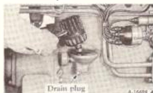
Illustr. 34 Removing the dirty oil filter element
