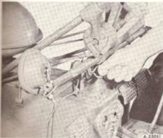
Illustr. 11 Pulling the choke rod out.
