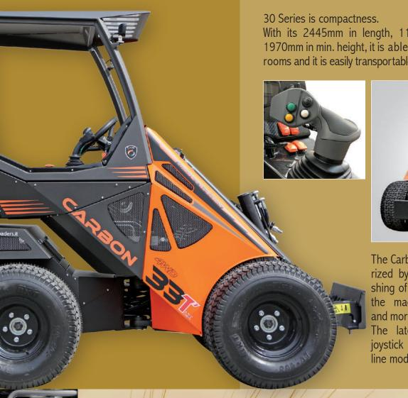
With its 2445mm in length, 1160mm in min. width and 1970mm in min. height, it is able to access the narrowest rooms and it is easily transportable.
