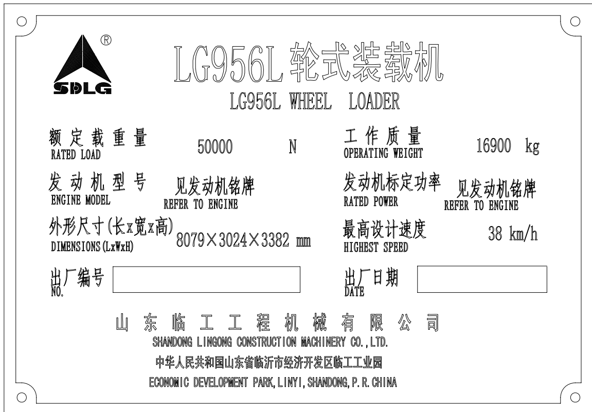
Figure 2-8 Nameplate of LG956L standard lift arm loader mounted with Shangchai and Cummins engine (with bucket of 3.0m 3 )
