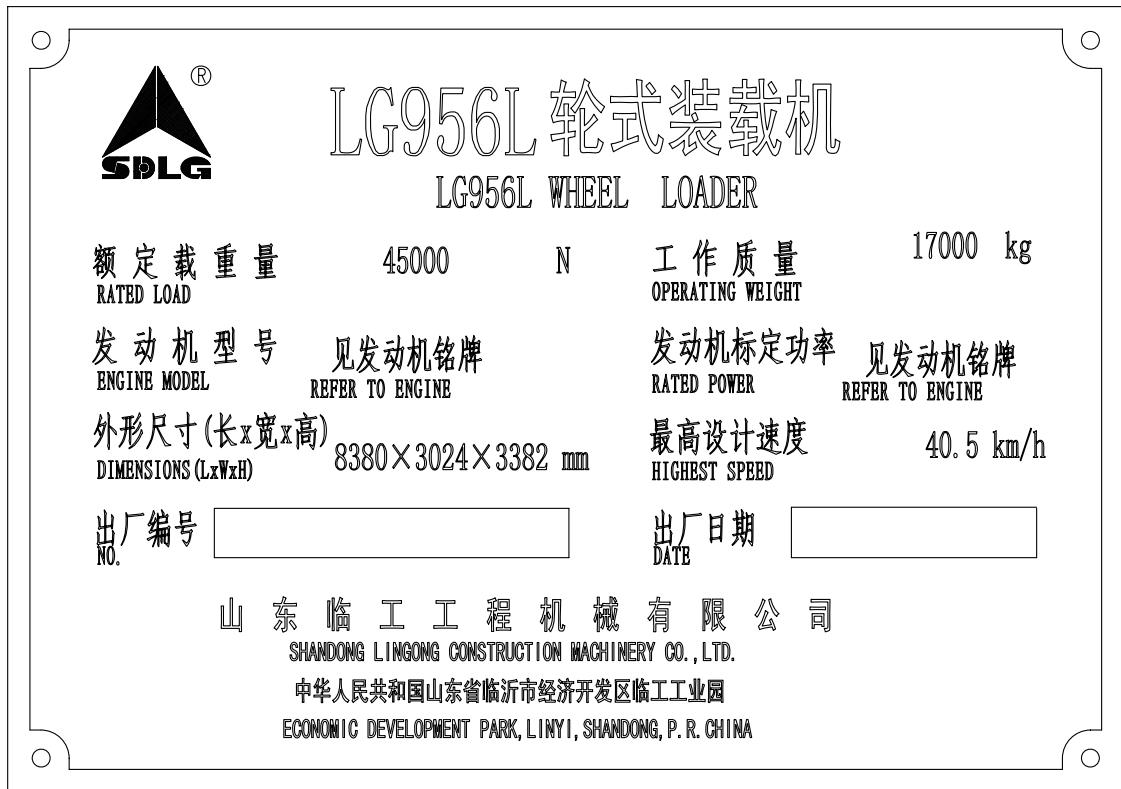
Figure 2-5 Nameplate of LG956L loader mounted with Weichai engine and long lift arm (with bucket of 2.7m 3 )
