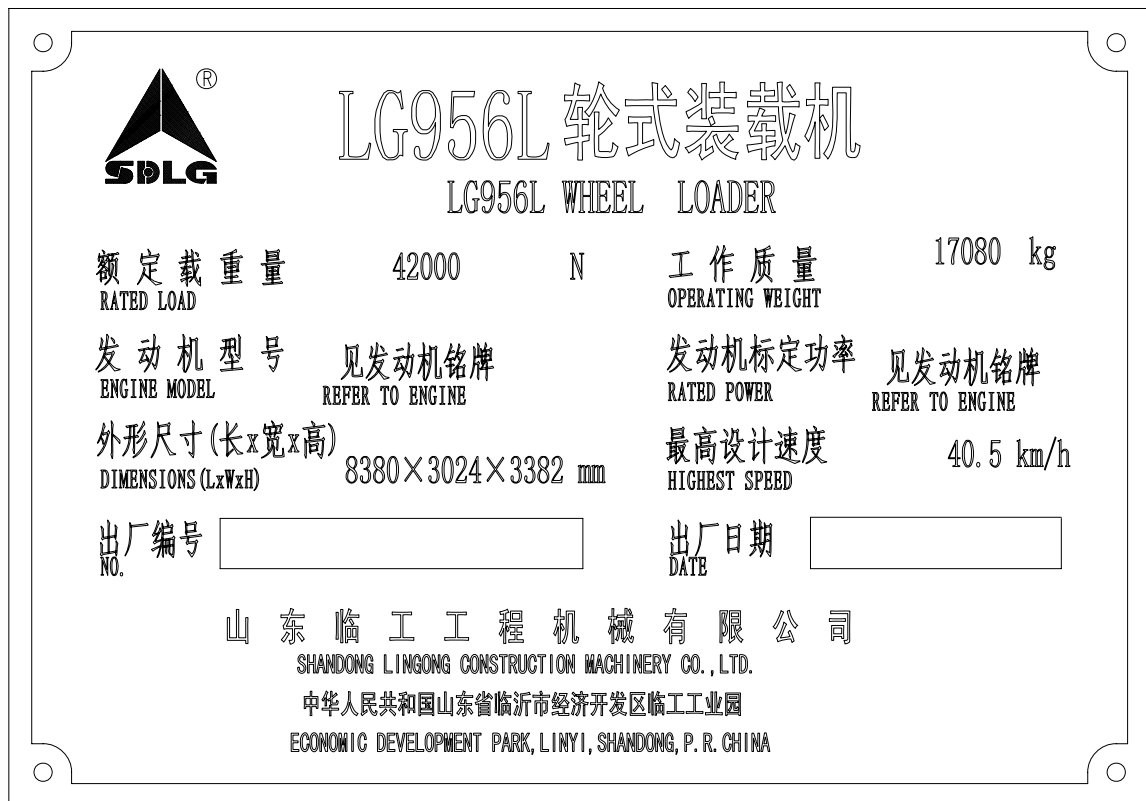
Figure 2-6 Nameplate of LG956L loader mounted with Weichai engine and super-long lift arm (with bucket of 2.7m 3 )
