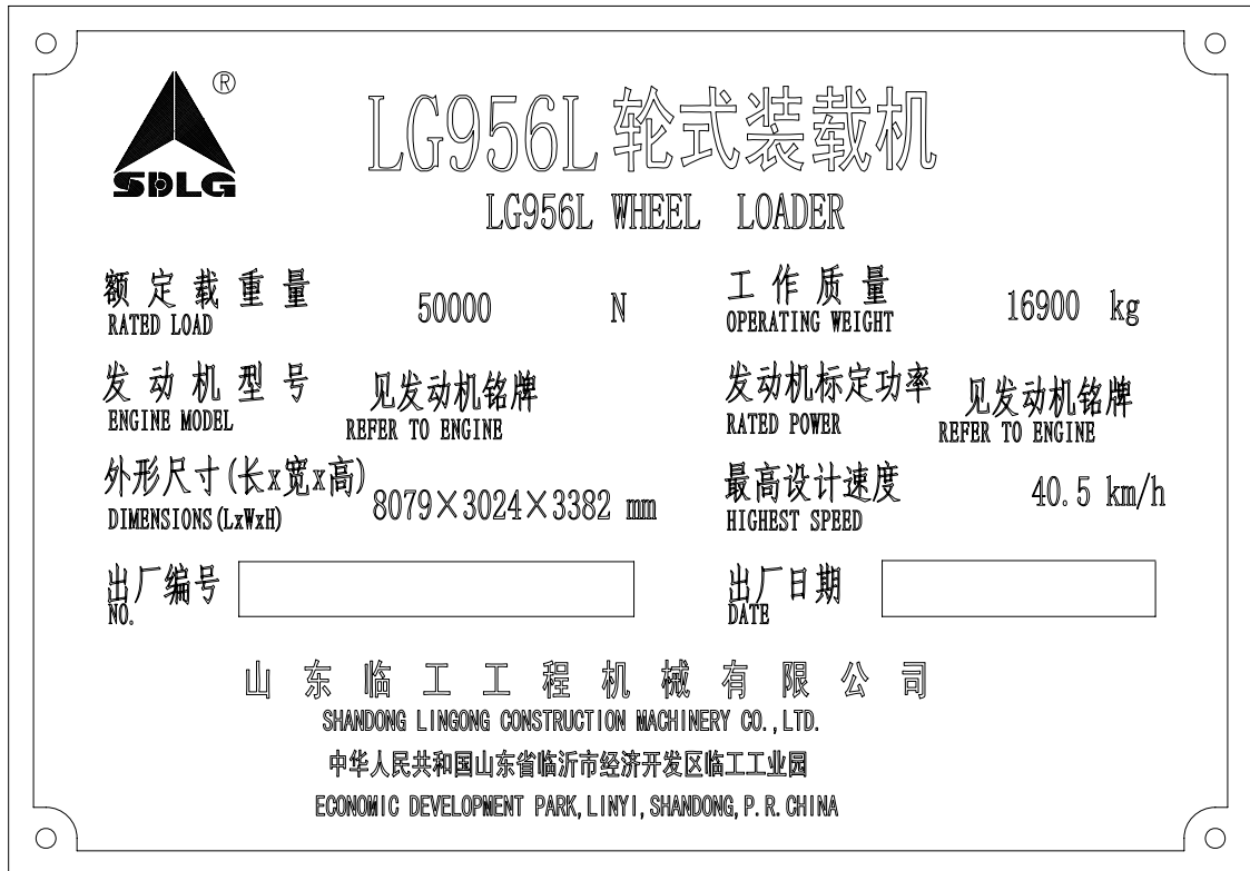
Figure 2-7 Nameplate of LG956L loader mounted with Weichai engine and standard lift arm (with bucket of 3.0m 3 )
