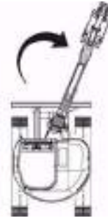
3 - pressing the pedal to the RH side swings the digger boom to the RH side.
