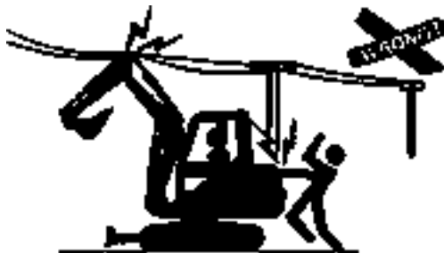
Electrical shock / electrocution
