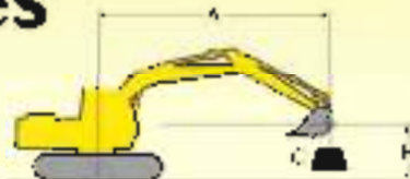
HD1430II 600mm Shoe, 6.15m Boom, 3.14m Arm, 1.4m 3 Bucket (1,140kg)
