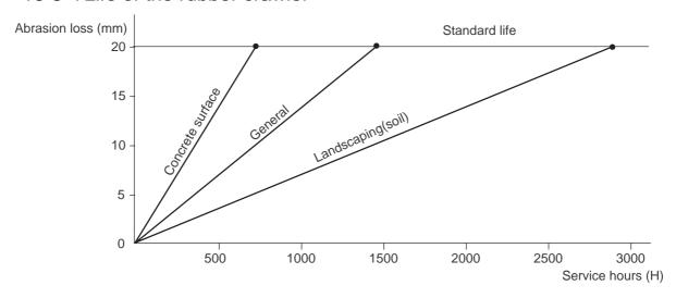
Check the remaining life of the rubber crawler by the abrasion loss in the rubber crawler height as shown in the figure below. Note that the life slightly differs depending on the conditions of site and the operation of the machine.
