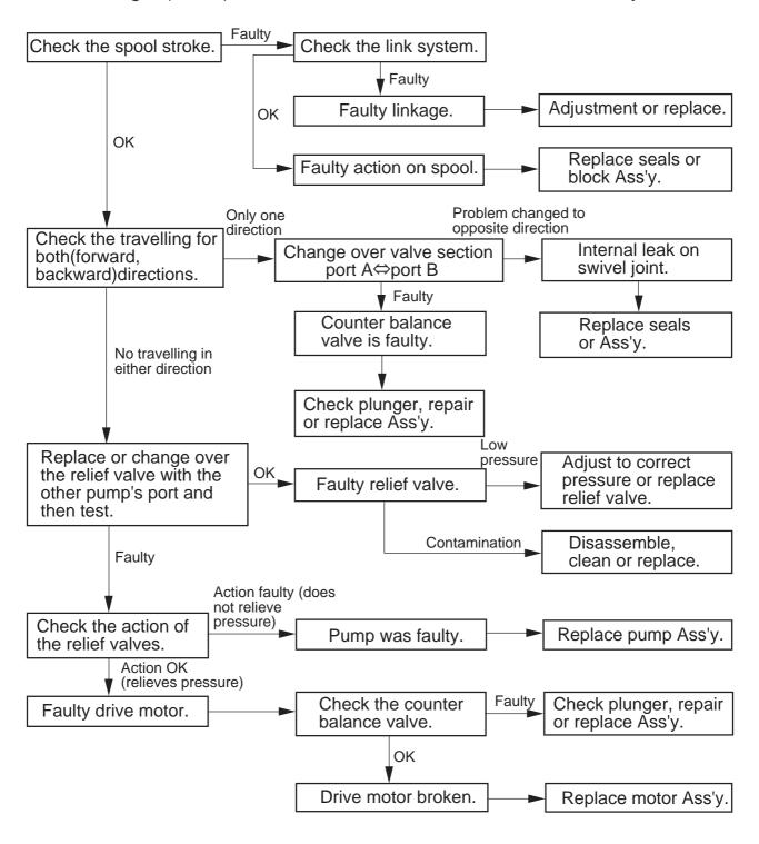
23-2-2 Travelling meander by slow speed on only right (left) hand side.
