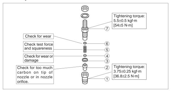
Disassembly sequence and inspection points
