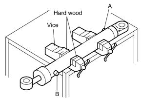
2. Loosen and remove the rod cover from the cylinder tube assembly with a hook wrench.
