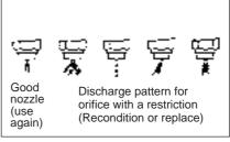
Orifice restriction test
