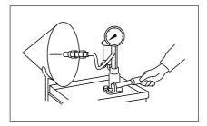
Fuel injection nozzle ready for test
