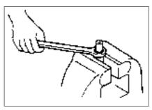
Removing tip from injection nozzle
