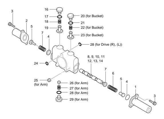
FOR BOOM/BUCKET/SLEW DRIVE(R)(L)/SWING P.T.O./DOZER/ARM
