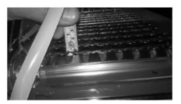
When keyboard pops-up you have to measure the lower sieve opening clearance and input the 1st value. Accept with OK button.
