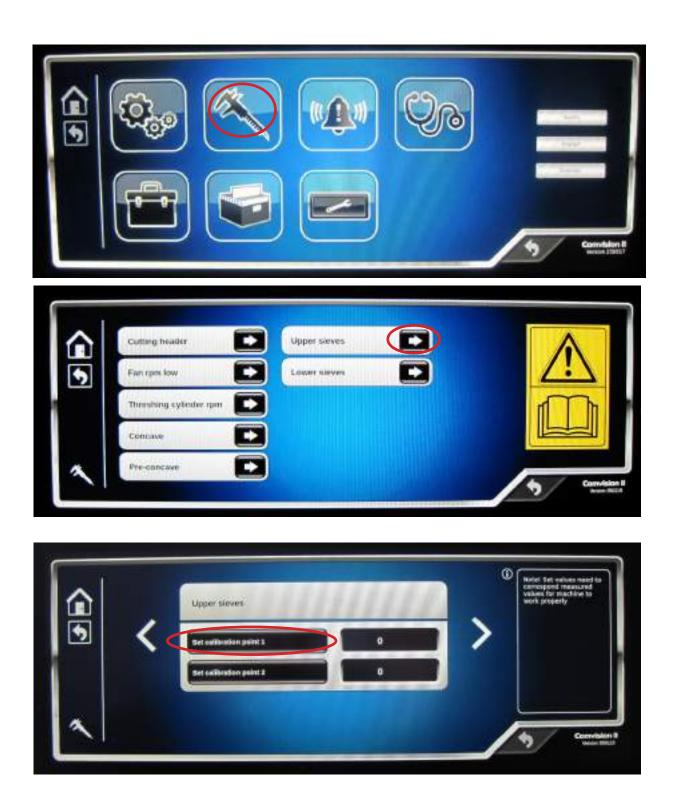
Operating actuator runs upper sieve to open and close positions automatically. And automatically calibrates those values.
