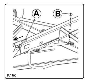
Drive the table above the trailer from the left-hand side so that the knife is level with the trailer marking sticks and brackets A at the rear of the table, fig K17, are between carriers B. Lower the table slowly. Make sure the table is positioned correctly: Reverse slowly so that the rear end of the table is against both the carrier limiters.
