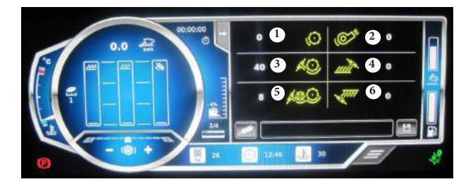
When pressing the value, new window will pop-up on the right side of the monitor. On this window you can adjust the selected value with arrow UP or DOWN. After adjustment, accept or reject the value with the buttons at the bottom of the window.
