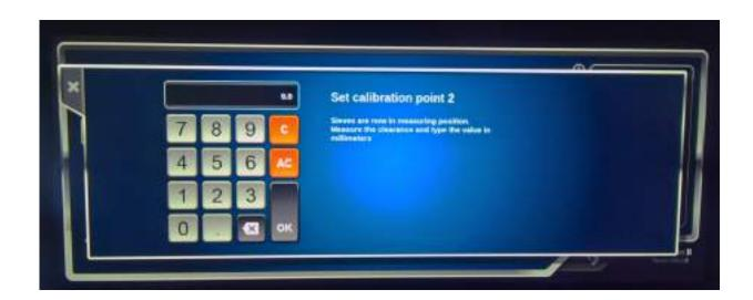
When keyboard pops-up again you have to measure the lower sieve opening clearance and input the 2nd value. Accept with OK button.
