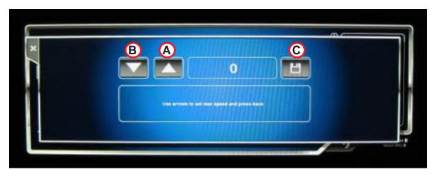
Push button (A) until fan speed doesn't raise anymore. Lower speed 50 units with (B) button. Save calibration value with (C) button.
