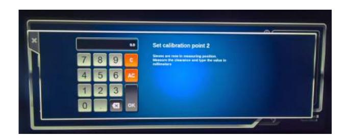
When keyboard pops-up again you have to measure the upper sieve opening clearance and input the 2nd value. Accept with OK button.
