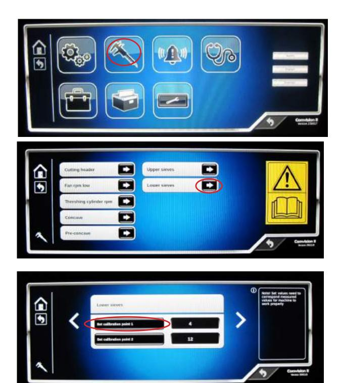
Operating actuator runs lower sieve to open and close positions automatically. And automatically calibrates those values.
