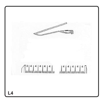
Attach the crop lifters with the knife finger fixing screw as shown in the figure. The numbers in the figure indicate the number of finger spaces. The crop lifters operate well if clearance to the ground is 8...10 cm, which clearance also prevents stone pick.
