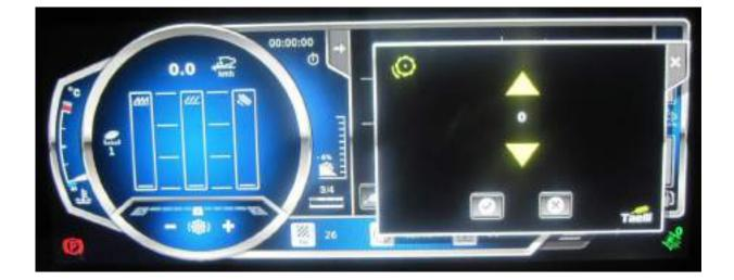
When pressing grain crop symbol at Harvesting adjustments window, "Taelli"- control system (OPTION) will popup. On this window you can make proper adjustments for different crops and then moving between them becomes more easy.
