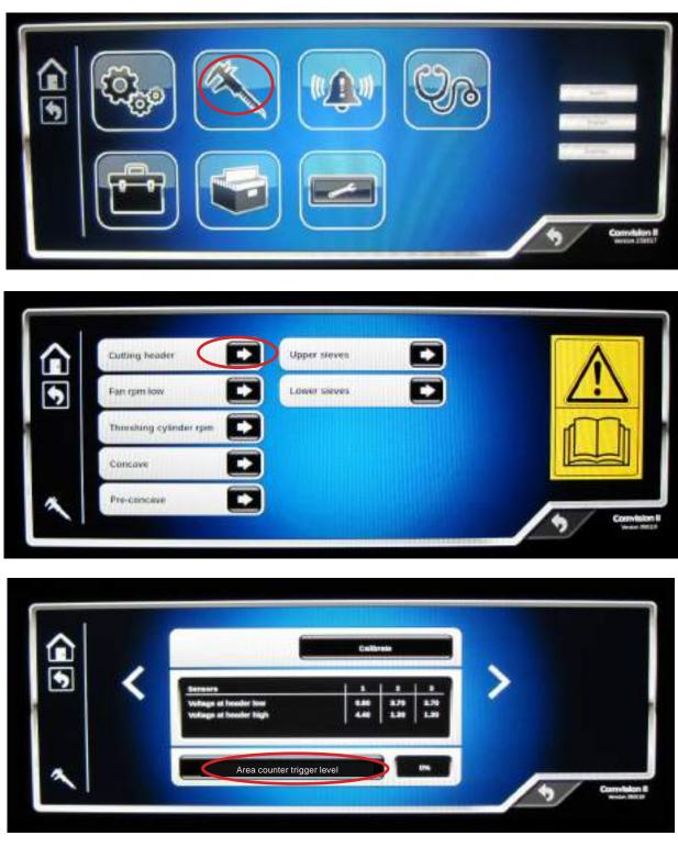
Adjust cutting header to height which you want hectare counter to activate/deactivate and push "save" button.
