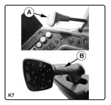
using lever B, fig. K7. With the lever in its mid position the combine is stationary if the gear is on and the engine running.
