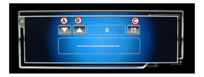
Push button (A) until fan speed doesn't lower anymore. Raise speed 50 units with (B) button. Save calibration value with (C) button.
