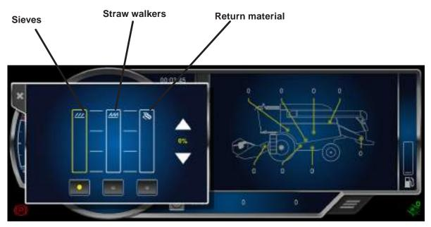
When pressing Harvesting adjustments at home page, new window will pop-up on the right side of the monitor. On this window you can adjust:
