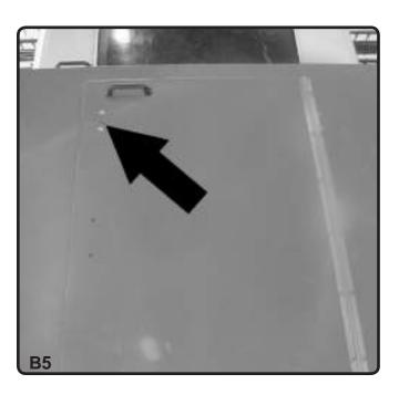
Open the locking on the grain tank cover, fig. B5, by placing the tool in the hole and turning counter-clockwise.
