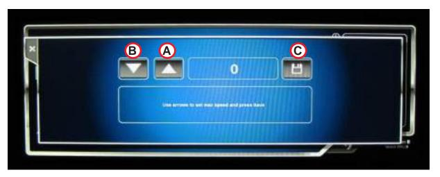
Push button (A) until threshing cylinder speed doesn't raise anymore. Lower speed 50 units with (B) button. Save calibration value with (C) button.
