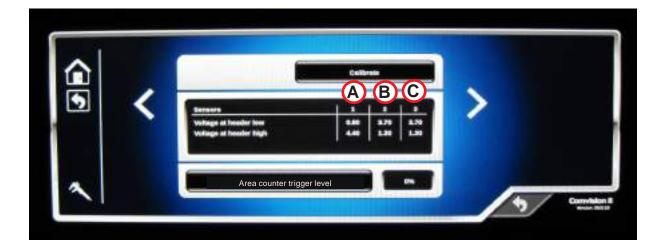
After calibration you can see the calibration values in columns. (A) Feeder house sensor. (B) Left hand side AHC sensor. (C) Right hand side AHC sensor. Values are Voltage values from sensors to cabin control unit when cutting header is down against ground and maximum up position.
