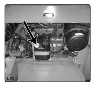
Be careful when handling DEF. DEF is aggressive to some materials and corrosive to some metals. DEF becomes crystalline when in contact with air. In case of a spillage rinse with plenty of water and dry with a clean cloth.
