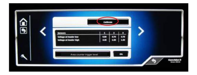
Make sure combine and cutting header are on flat surface. Lower cutting header down on the ground. Push and hold down cutting header lowering button together with rising button. Hold buttons on the bottom until calibration starts and header begins to rise. Release buttons and wait until cutting header stops moving and calibration ends.
