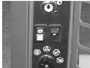
Figure 2 Parking Brake Switch
