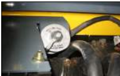
Figure 14 – Battery Disconnect Switch
