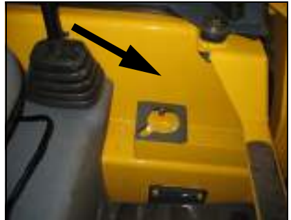
Figure 1 – Fire Extinguisher Location
