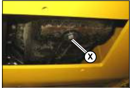
Figure 94 – Engine Oil Drain Plug
