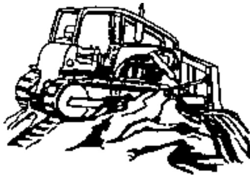
Fig. 4.34. Slope Edge Operation
