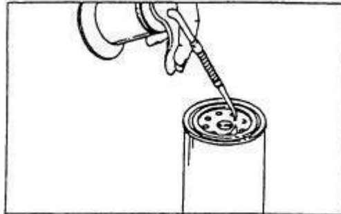
Fig. 5.23. Preparation of Coolant Filter for Replacement
