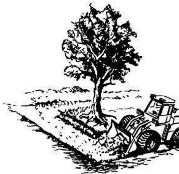
Fig. 4.56. Removing Large Trees
