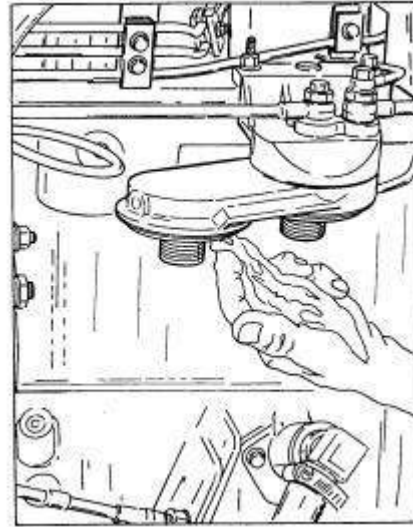
Fig. 5.31. Cleaning Fuel Filter Header
