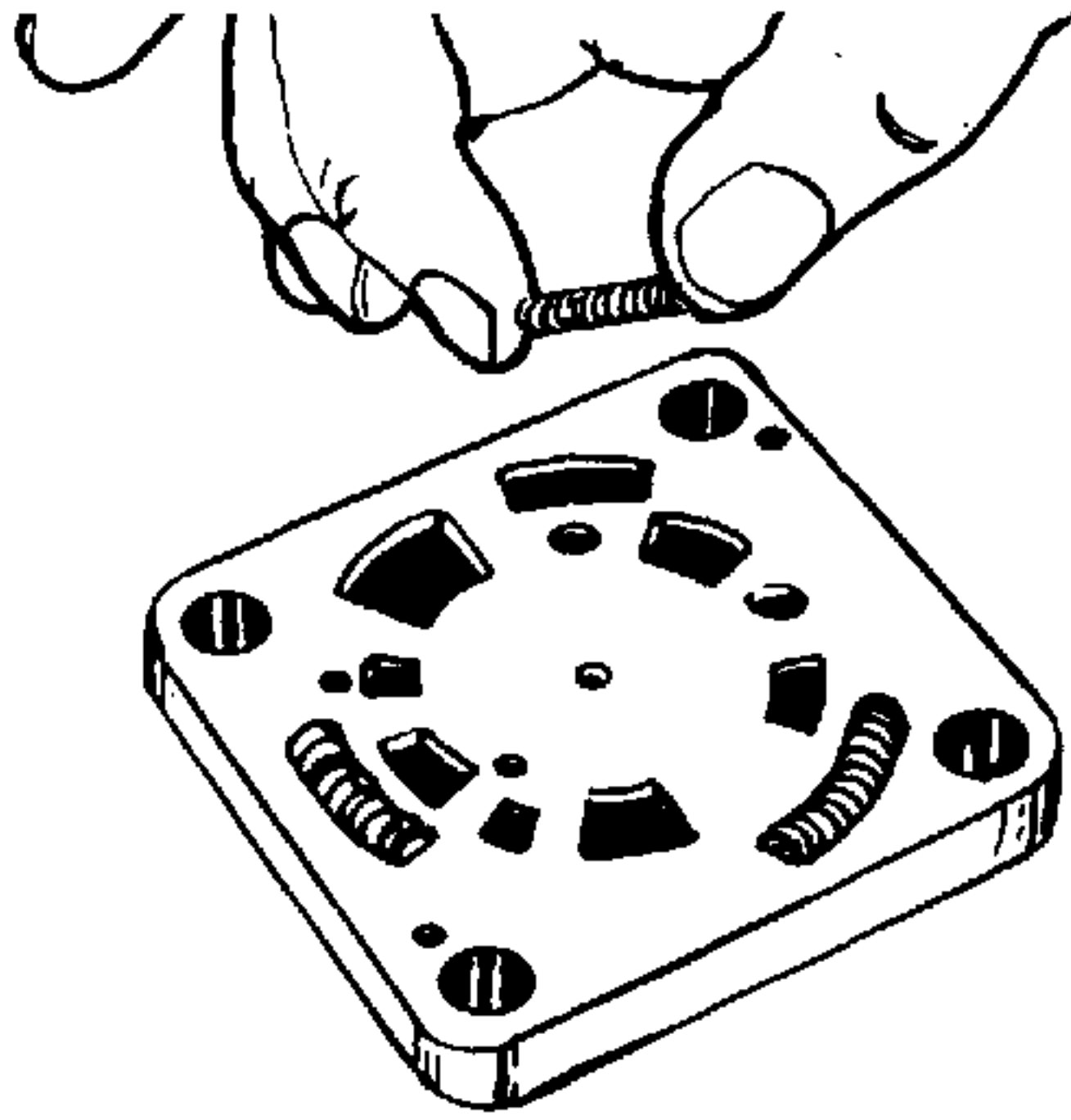
Figure 4-85. Installing 3/4-inch Springs.
