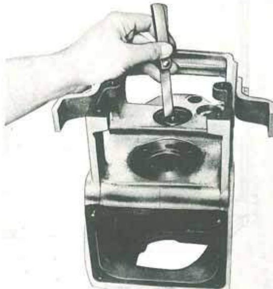
Illust. 2-49. Measuring snap ring groove gap.
