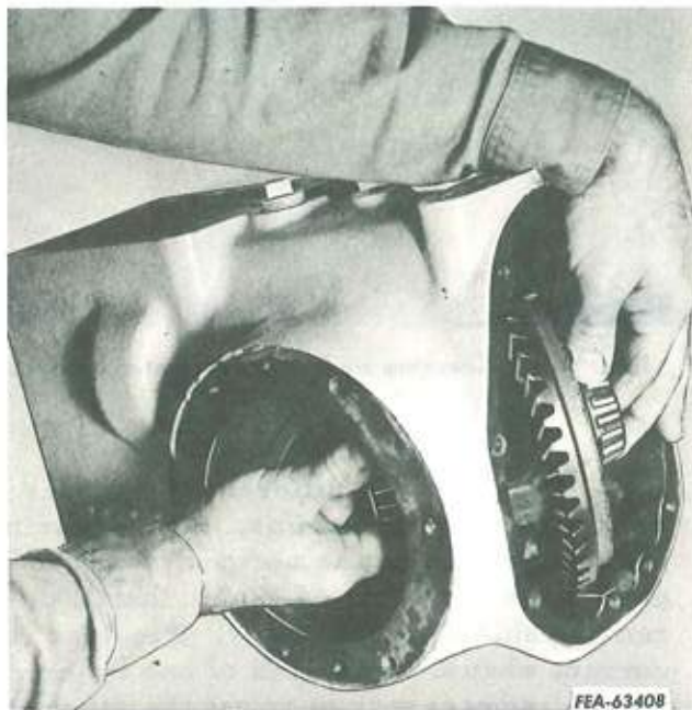
Illust. 2-41. Removing differential from the transmission case.
