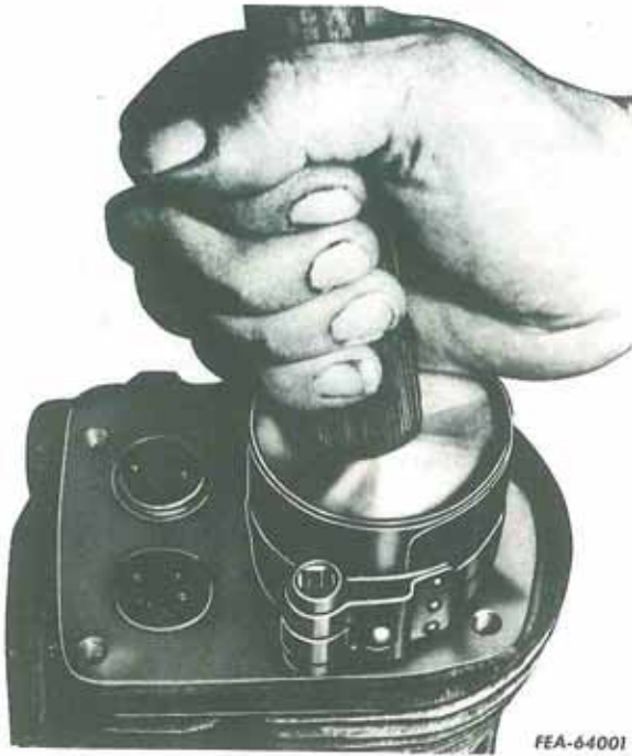
Illust. 1-14. Installing piston assembly.
