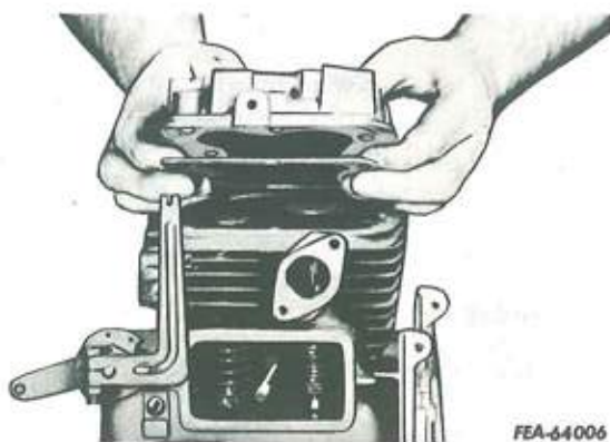
Illust. 1-19. Cylinder head assembly.
