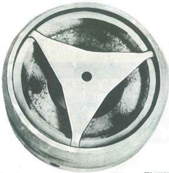
Illust. 2-58. Pressure spring located on pulley.
