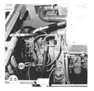
Ignition key in position "ZERO". Remove connector (9) from load limit regulator valve or connector (9a) from the electronics box.
