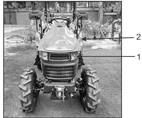
1. Head Light 2. Turn Signal Light
