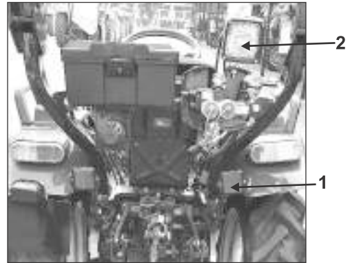
1. Rear Reflection Light 2. Plough Light
