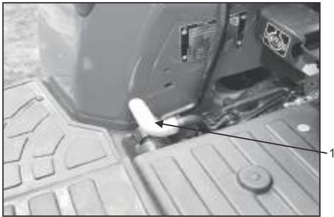
1. Differential Lock Pedal
