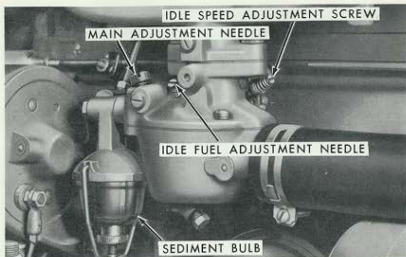
Figure 32 Adjusting the Carburetor (Series 2000)
