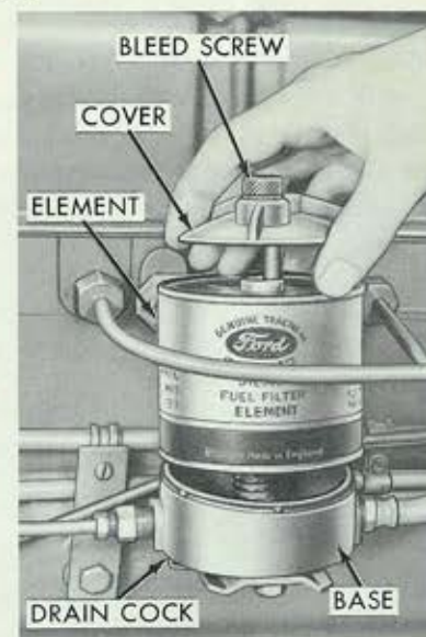
Figure 25 Replacing Diesel Fuel Filter
