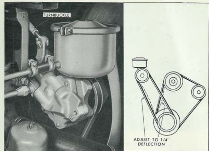
Figure 31 Adjusting Fan, Generator and Power Steering Pump Belts
