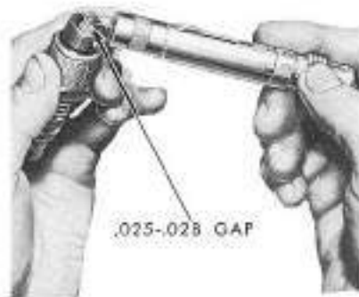
Figure 36 Checking Spark Plug Gap
