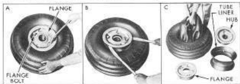
Figure 47 Single Front Wheel Tire Removal
