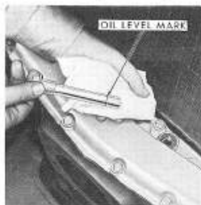
Figure 25 Checking Pedestal Oil Level
