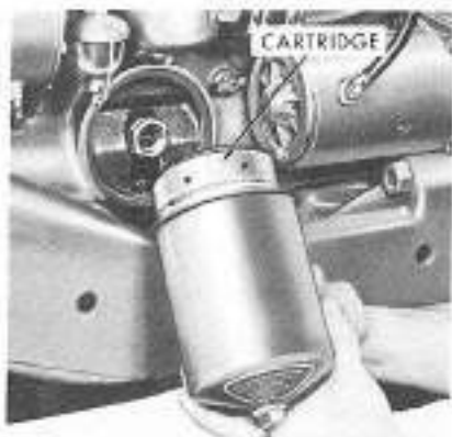
Figure 27 Replacing the Oil Filter Cartridge
