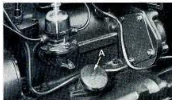
FIGURE 2/3. ENGINE OIL FILLER (early tractors) A. Filler cap and dip stick
