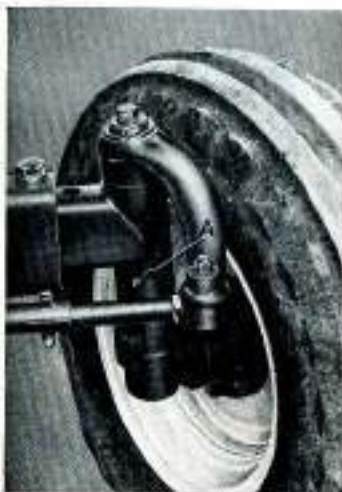
FIGURE 3/12. FRONT AXLE A. King pin lubrication point
