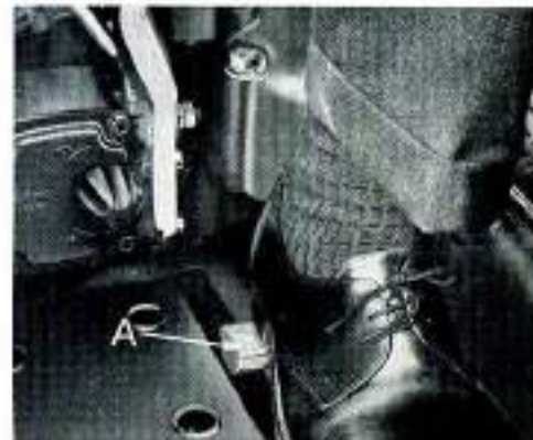
FIGURE 1/18. DIFFERENTIAL LOCK A. Pedal
