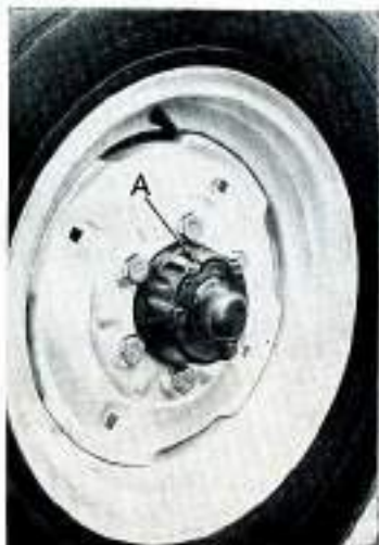
FIGURE 3/13. FRONT HUB A. Front hub greaser (fitting)
