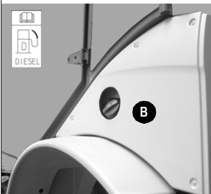
Fig. 156: Additional tank fuel filler inlet
