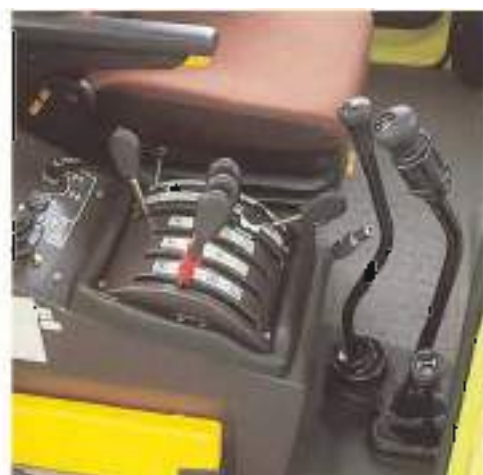
The control levers for the transmission, hydraulic system, all wheel drive and differential locks are on the right-hand side of the driver's seat.
