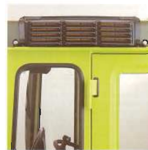
Large filtering capacity that the three-stage fan delivers dust-free air. An air conditioner is optional.
