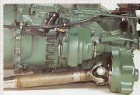
The rear axle drive shaft.
