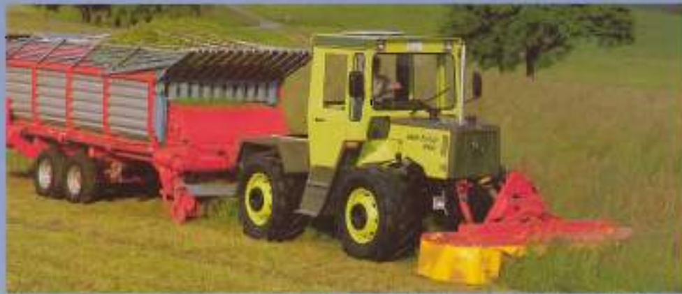
With a front loader and self-loading trailer, the MB-trac becomes a "roll-over express" - a classic combination for zero grazing or one-man silage harvesting.
