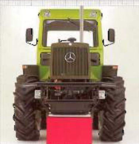
The hub-reduction axes provide high ground clearance – essential for row crop work.
