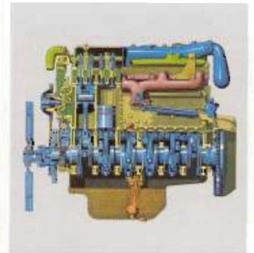
The OM 352 engine in the MB-trac 1000 is distinguished by its low fuel consumption and smooth 6-cylinder performance.
