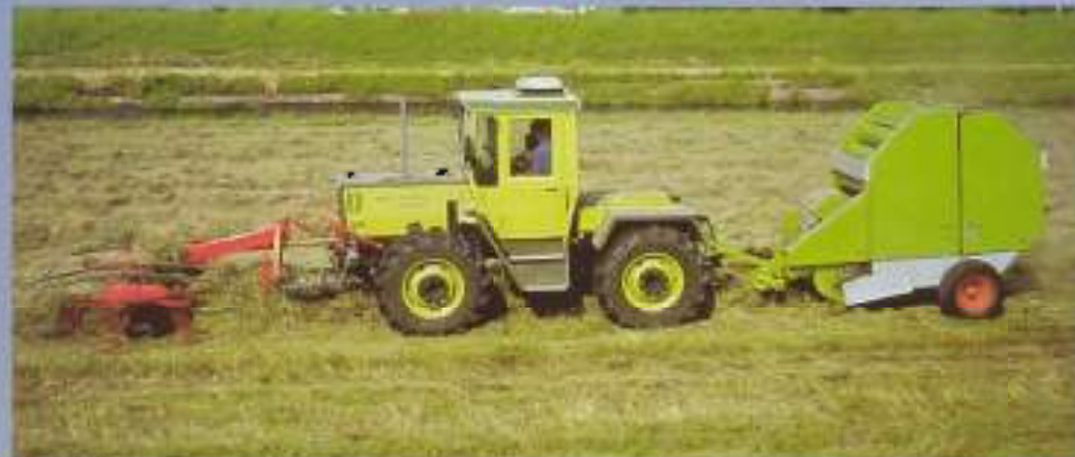
With front-mounted sweepers, the windrowing is not disturbed over, thus giving a cleaner pickup, windrowing does not get ahead of the baler and two jobs are done in one pass.
