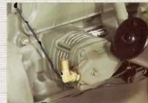
The maintenance-free and reliable engine-mounted compressor provides auxiliary power for the braking system.
