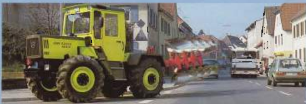
With 4 wheel brakes, front spring axle and plenty of front end weight, the MB-trac can be driven on paved roads with heavy fully mounted ploughs with complete safety.
