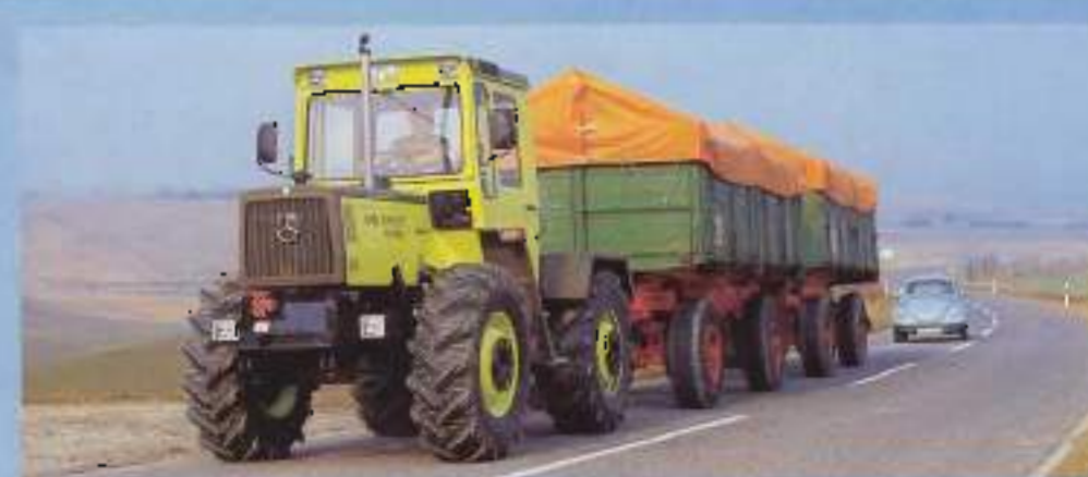
Because of its four-wheel braking system the MB-trac can be stopped quickly and with low pedal pressures, even in critical situations.
