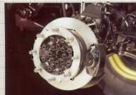
The MB-trac has seven pneumatic hydraulic brakes on all four wheels and because they are externally mounted they are very easy to service. A further advantage, normally only available on heavy cars, is a brake wear indicator.
