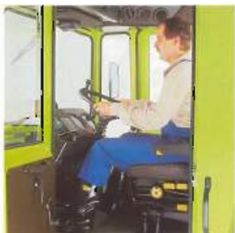
The comfortable seat which is equipped with spring suspension and hydraulic damping is adjustable in six directions, including the back rest and seat cushions, as well as seat height and fore and aft adjustment.
