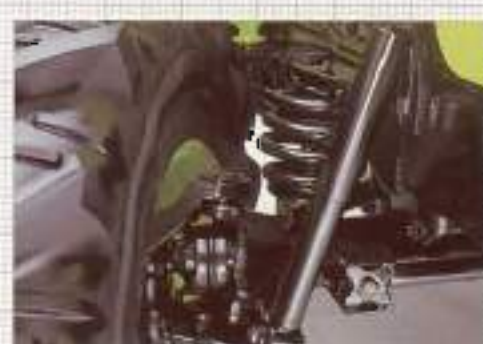
The strong rear axle absorbs heavy bumps and the shock absorbers prevent bounce. With such suspension there is also more lateral support, making it safer when crossing ruts than with a conventional coil-over axle.
