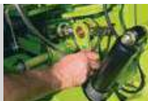
Mechanical shear bar adjustment
