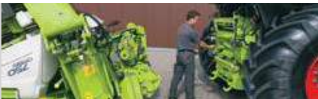
Ease of access to knife drum
