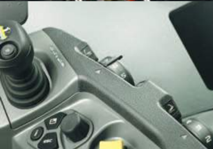
External controls for the front linkage and one spool valve
