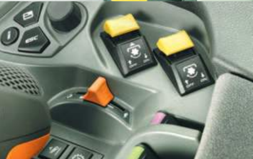
External controls for front and rear PTO
