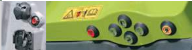
External controls for front and rear PTO
