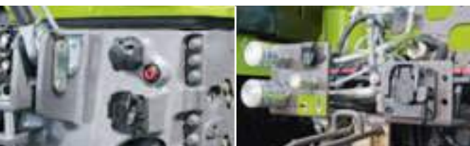
ISOBUS connections at the front and rear
