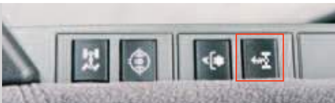
Switch to activate front axle suspension
