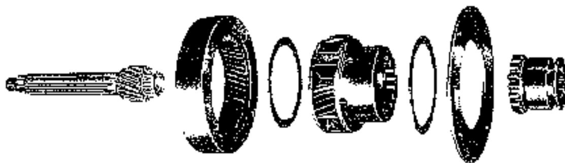
Fig. 191. - Epicyclic reduction components.
