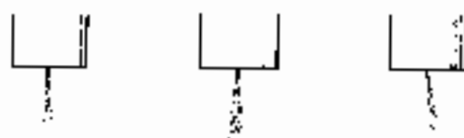
Good Bad Bad Spray patterns in chattering test
