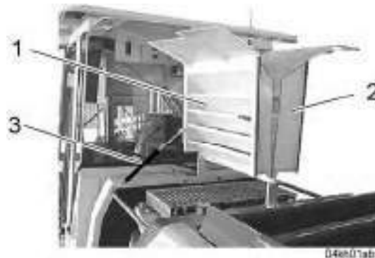
Cooling system hood
