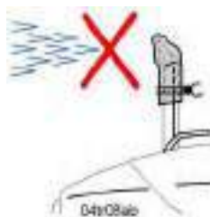
Blocking off the exhaust pipe opening
