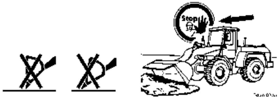
Impermissible bucket positions
