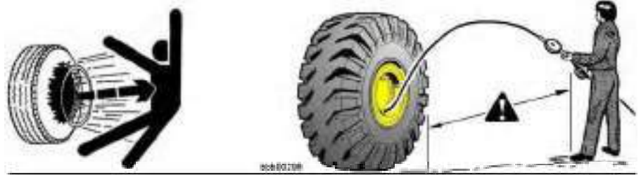
Checking and adjusting the tyre pressure
