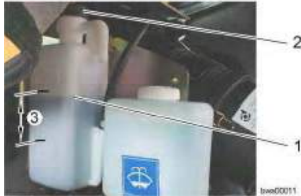
Checking the coolant level
