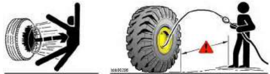
Checking and adjusting the tyre pressure
