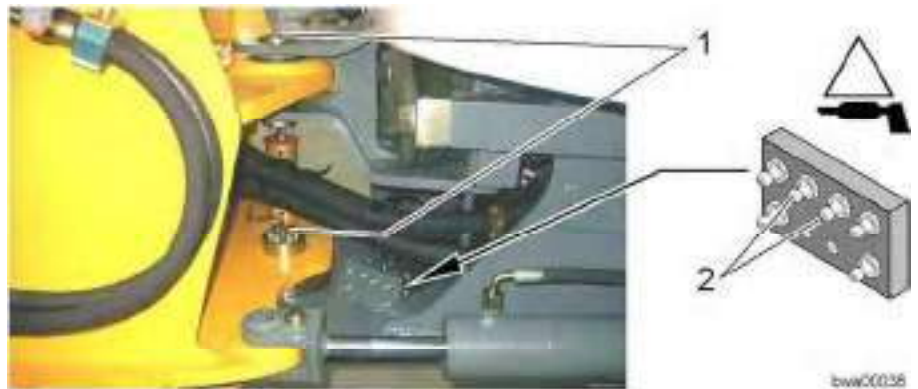
Lubricating points on the articulated oscillating bearing and the rear oscillating bearing
