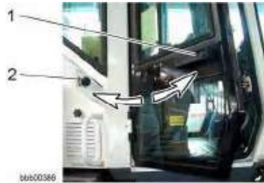
Opening the emergency exit
