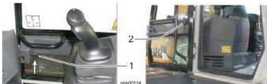
Opening the emergency exit
