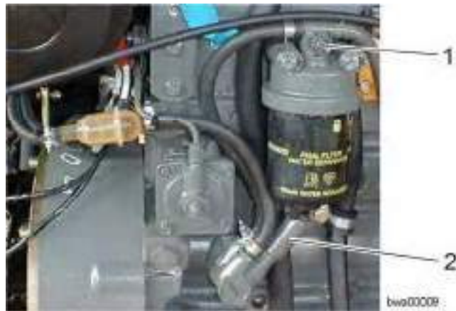
Bleeding the fuel system
