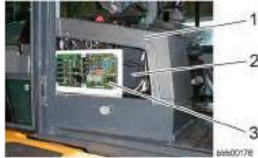
Fuse box with A4 control board
