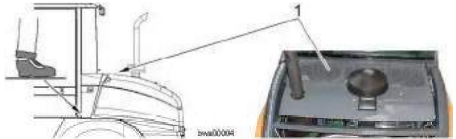
Cooling system grille
