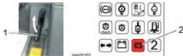
Display unit and parking brake switch
