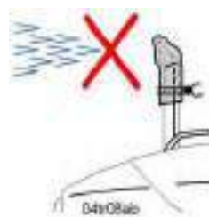
Blocking off the exhaust pipe opening
