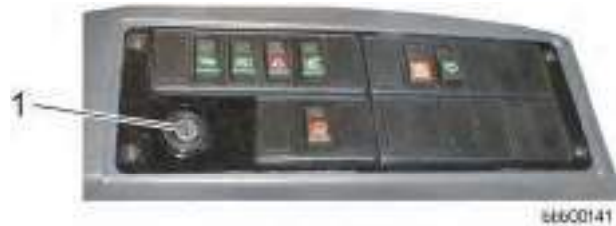
Ignition switch position
