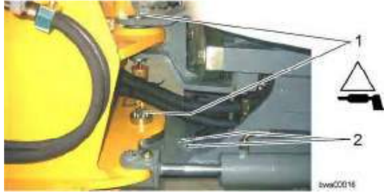
Lubricating points on the articulated oscillating bearing and the rear oscillating bearing
