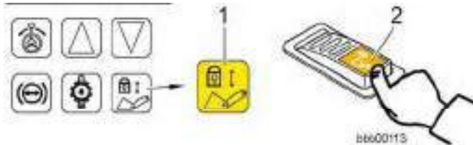
Working hydraulics lockout
