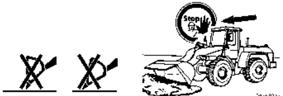
Impermissible bucket positions
