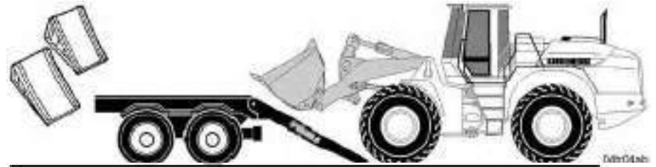
Loading the machine
