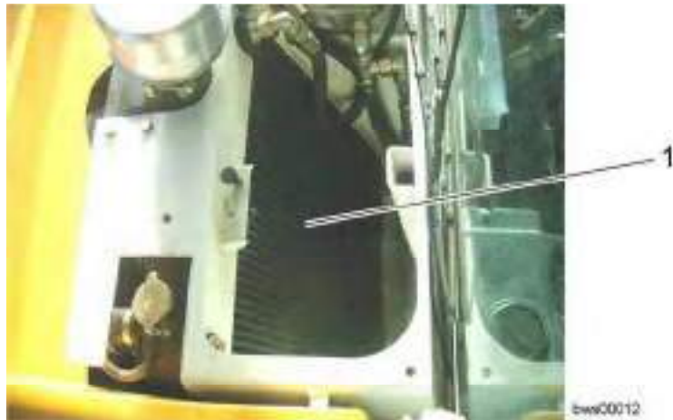
Cleaning the cooler units
