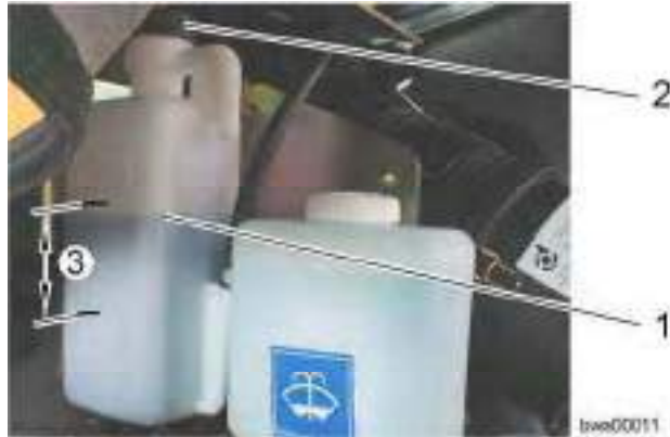
Checking the coolant level
