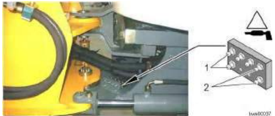
Lubricating points on the rear axle kingpin bearings
