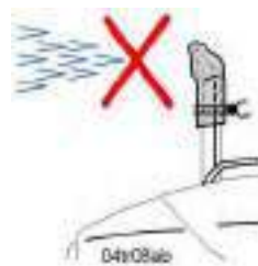
Blocking off the exhaust pipe opening
