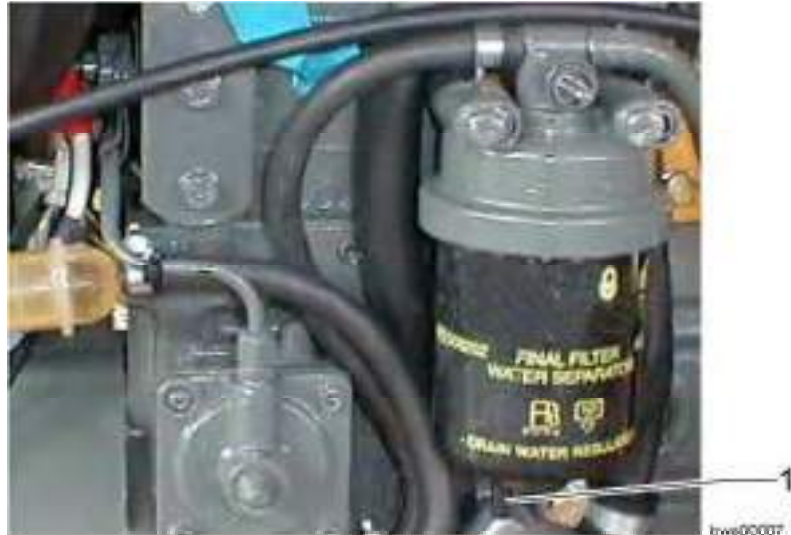
Draining off condensate
