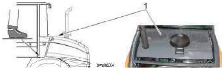
Cooling system grille
