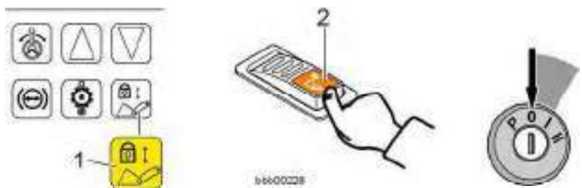
Working hydraulics lockout
