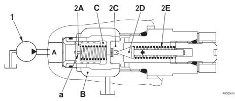
• If abnormal pressure is generated in the circuit or the shuttle valve of HST motor is at neutral and the oil pressure at ports A and C reaches the pressure set by spring (2E), poppet (2D) is pushed to \_\_\_\_ direction, and oil at C is relieved to port B and pressure of the oil at C reduce.
