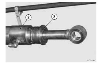
4 - Unscrew the head (3) and extract it completely from the cylinder (2).
