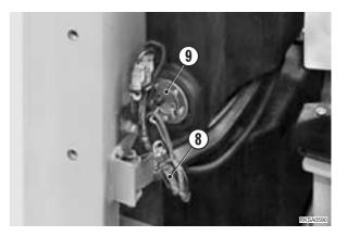
6 - Disconnect the fuel level sensor connector (8).
