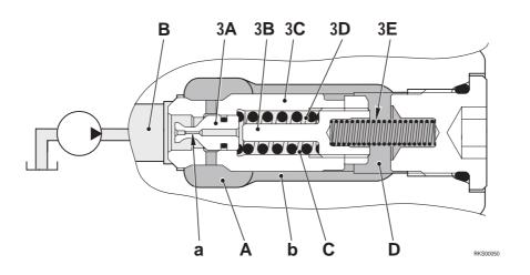
If abnormal pressure is generated in the circuit and the oil pressure at ports A and D reaches to the pressure set by spring (3D), poppet (3A) is pushed to \_\_\_\_ direction, and oil at port A is relieved to port B to reduce the oil pressure at port A.
