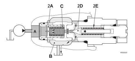
• When the pressure of the oil at port C goes down, a differential pressure is occured between ports A and C because of orifice a in valve (2A).
