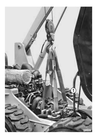
5 - Loosen the eight screws (12) and remove the pump (1) complete with the flange (13).
