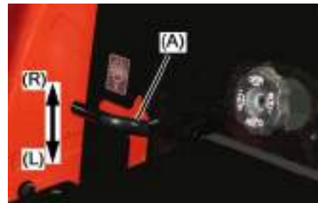
(A) Differential lock pedal (R) Release lock (Release pedal) (L) Apply differential lock (Depress pedal)
