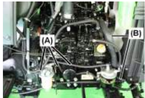
(A) Fuel pipe (B) Radiator hose
