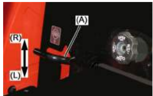
(A) Differential gear lock pedal (R) Release lock (release pedal) (L) Lock differential gear (keep depressing pedal)
