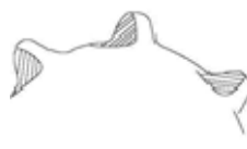
Wear condition of driving sprocket
