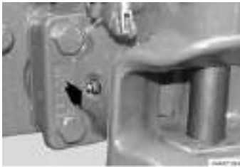
Automatic trailer hitch with cylinder-type bolt.
