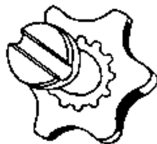
Fig. 26—When properly assembled, slot in end of drive link must align with valley of inner gear as shown to provide correct valve timing.
