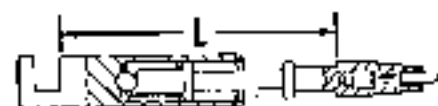
Fig. 169—Collapsed length (L) of pilot control valve should be 102.75-103.12 mm (4.039-4.060 inches) measured as shown. Length is adjusted by installing a different diameter spacer ball.
