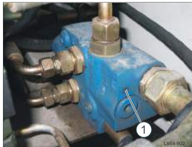
Fig. 83 "LSD" (ride control system) pressure reduction
