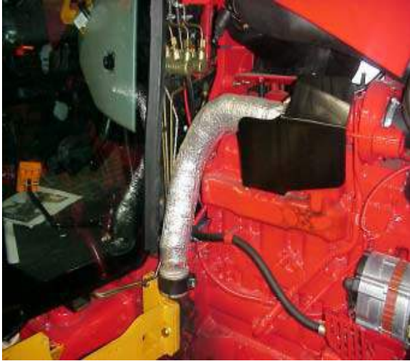
Factory Exhaust Pipe Removed
