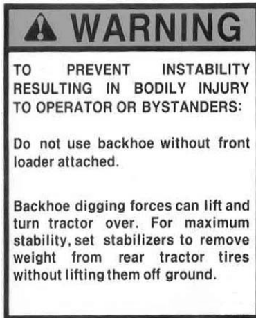
Warning BH35-0105 Location : Main valve cover
