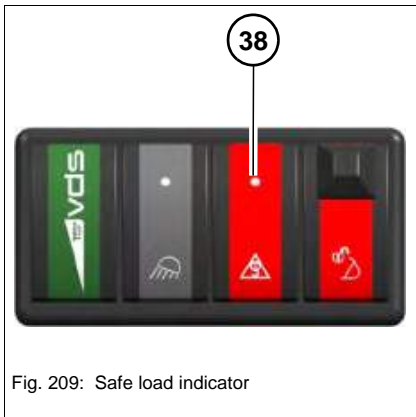
Fig. 208: Safe load indicator light
