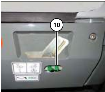
Fig. 241: Lubrication point of ball bearing race
