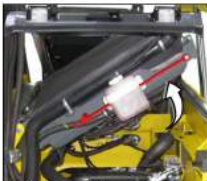
Fig. 12: Raising the radiator
