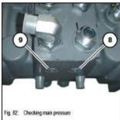
Fig. 81: Checking main pressure
