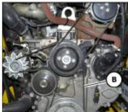
Fig. 66: Checking V-belt tension
