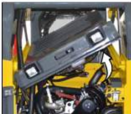
Fig. 13: Raising the radiator
