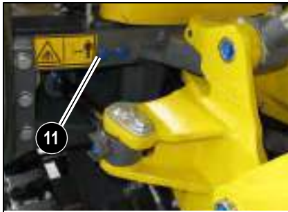
Fig. 49: Lubrication points of ball bearing race
