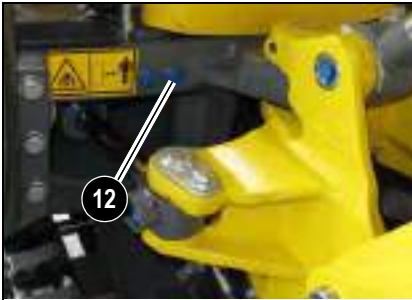
Fig. 51: Teeth lubrication point
