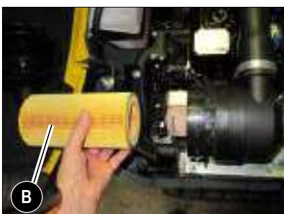
Fig. 22: Removing the outside air filter
