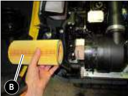
Fig. 24: Removing the outside air filter
