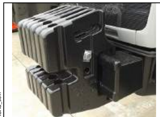
1 – Ballast holder 2 – Ballast elements
